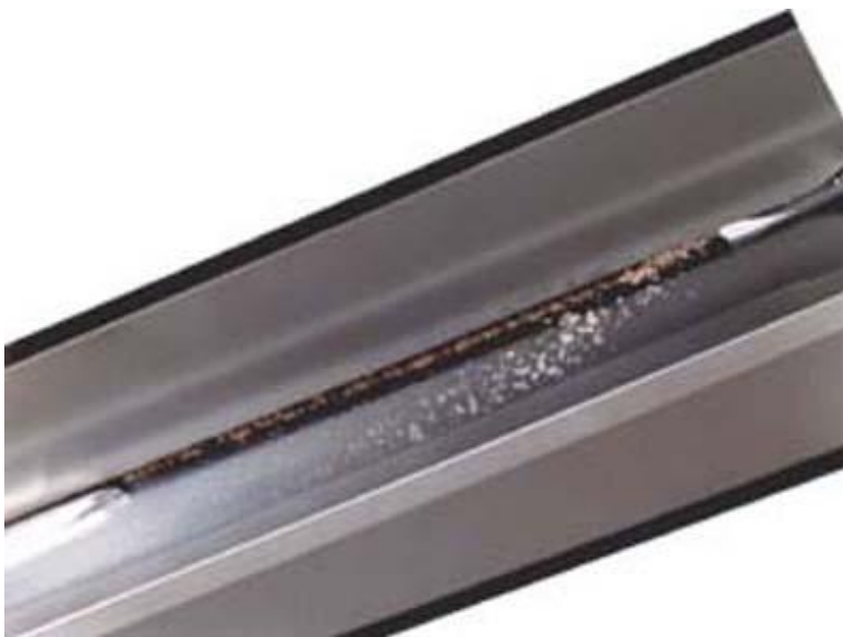
Figure 3.: Separation by exploiting paramagnetic susceptibility is shown here. The mixture is fed into the anadynamic region inside the gap of the LB-1. The magnetic system is inclined so that gravitational force urges particles toward the near side of the chute. The darker paramagnetic grains can be seen moving along the magnetic barrier, while the light-colored diamagnetic grains pass through it. The sample is the same mixture of diamagnetic and weakly paramagnetic grains used for the separation shown in Figure 1.
